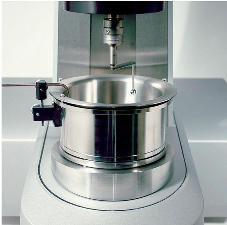
REOMETRO A SFERA ROTANTE BMS (Ball Measuring System)
